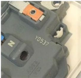
Figure 5 - Date coding on a wiring accessory showing week 46 of 2007
