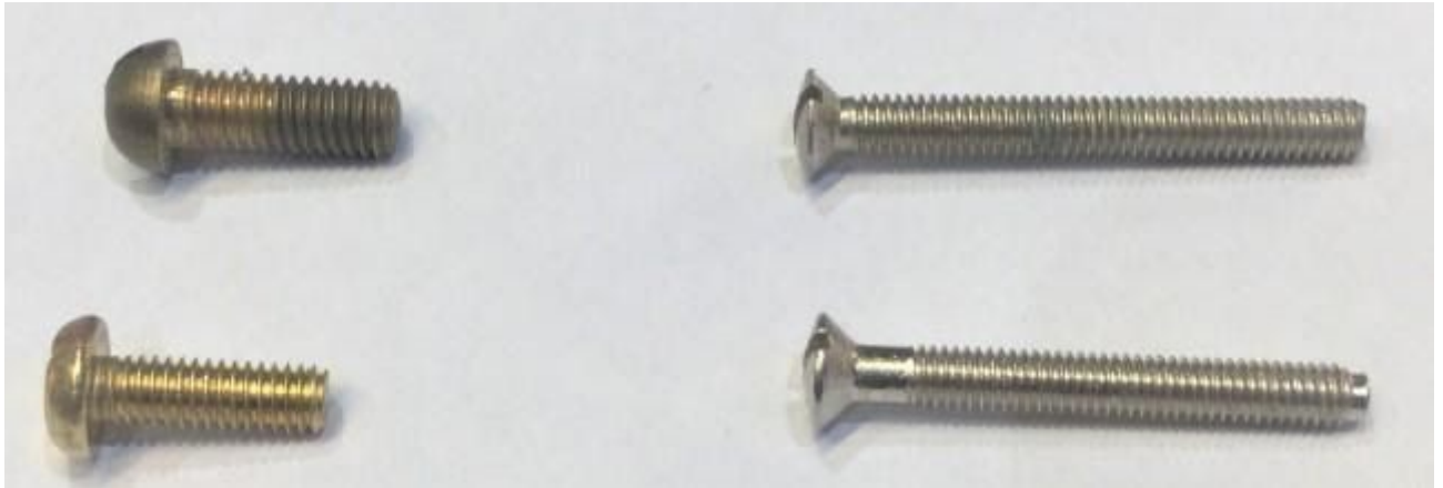
Figure 2 - Common fixings screws (Imperial version shown on top with its metric counterpart beneath)
