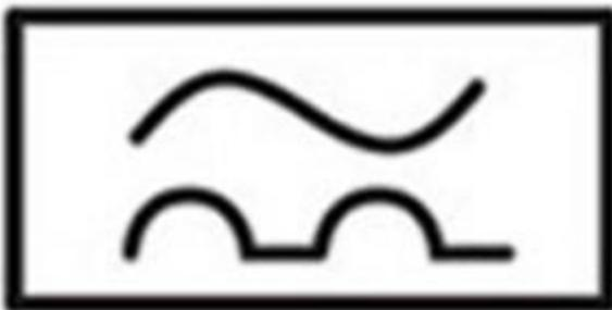
Type A RCDs are used for alternating sinusoidal residual current and for residual pulsating direct current up to 6 mA.
